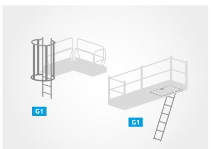
• A modular access ladder integrated with formworks, for access to a platform for concrete works, and for screwing formworks together (on one side) (G1)
